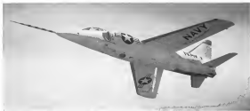
VENTED WING of rolling Tiger is created by mixed spools on upper surface of wing and restricted gaps on lower surface.
